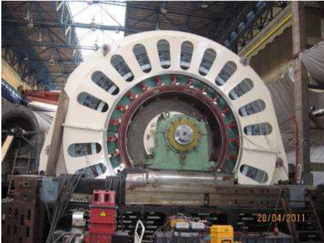
Figure 7. Direct Current 5500 kW engine which is a part of INCO delivery, Source: www.incoengineering.cz
